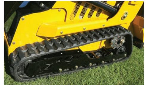
**ADAPT TO THE CHALLENGE.** With a universal mounting plate, option of 7 in (17.8 cm) or 9 in (22.9 cm) tracks and multiple engine options to choose from, the S925TX has the options to help increase productivity on the job.
